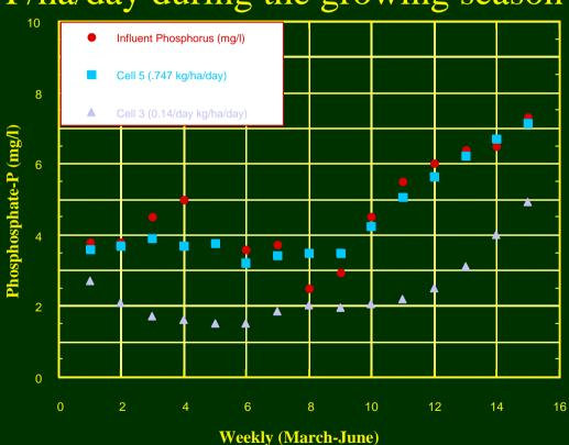
Seasonal Phosphorus absorption and release-blue dots represent tap water in wetland that received secondary effluent-orange dots represent a lower P load-phase shift but phosphorus returns to about 90% of influent in non-growing season
